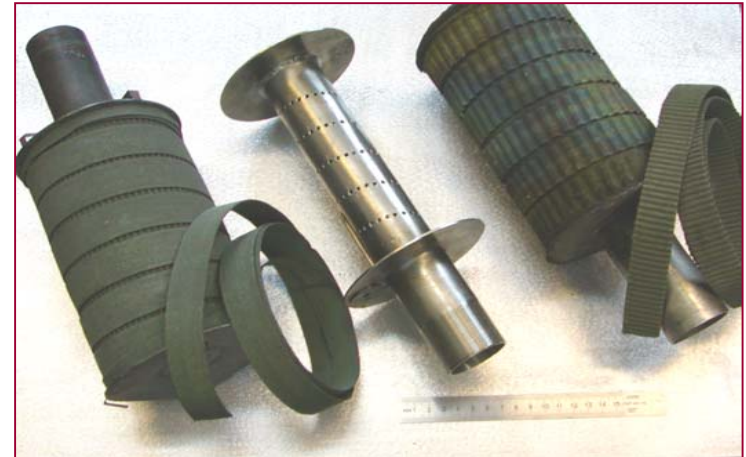
Tape catalyst reactor of the syngas capacity ca. 5 m 3 /hour
