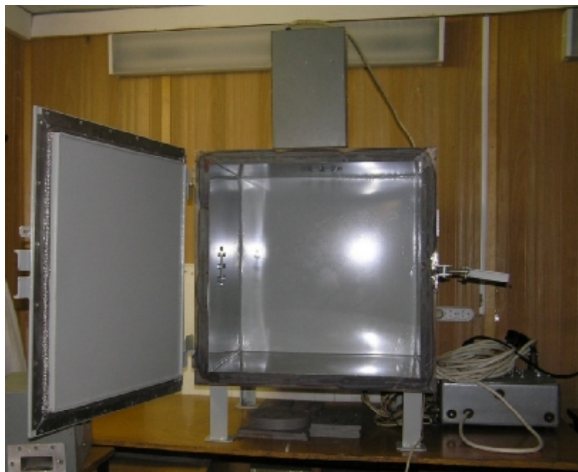
Fig. 3. Photo of the microwave chamber for pilot studies of temperature distribution in the volume of the material.
