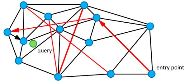
**Fig. 1.** Graph representation of the structure. Circles (vertices) are the data in metric space, black edges are the approximation of the Delaunay graph, and red edges are long range links for logarithmic scaling. Arrows show a sample path of the greedy algorithm from the entry point to the query (shown green). (For interpretation of the references to color in this figure legend, the reader is referred to the web version of this article.)
