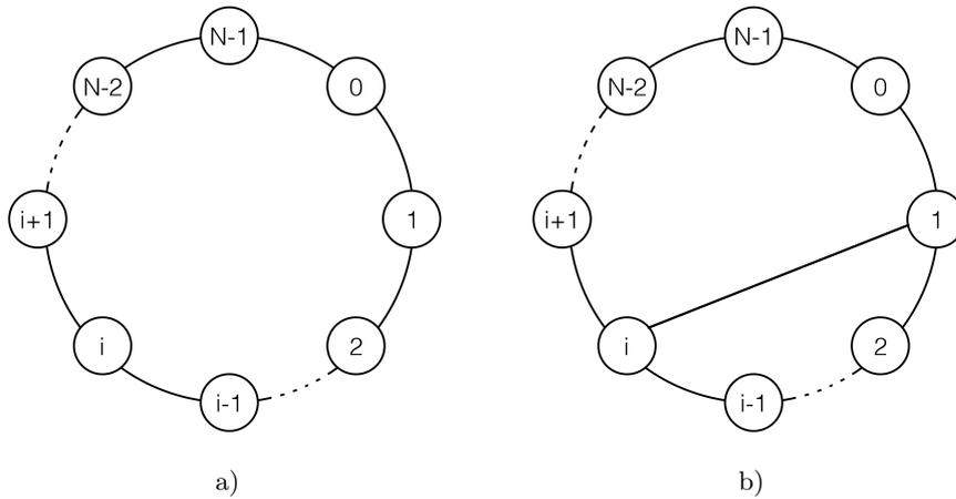
**Fig. 2.** a) Regular communication topology. In this topology all communications are local. b) Small-world communication topology. Besides the local communications, there are additional distant communications. The  $LP_1$  and  $LP_i$  are distant processes, connected by a communication link.
