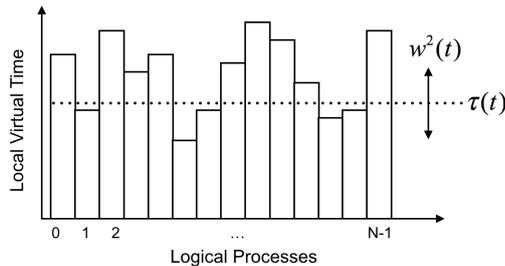
**Fig. 1.** A snapshot of local virtual time profile at a simulation step  $t$ . The LPs have their values of the LVT.  $\tau(t)$  is a local virtual time averaged over all logical processes and  $w^2(t)$  is an average squared width of the profile.
