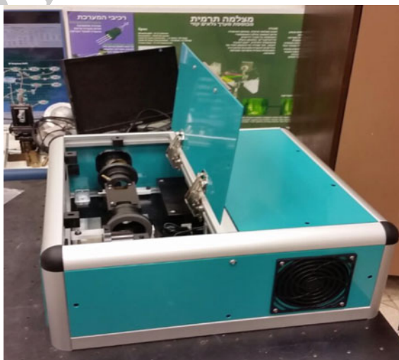
Fig. 2 An in vitro MIR-ATR spectroscopy system
