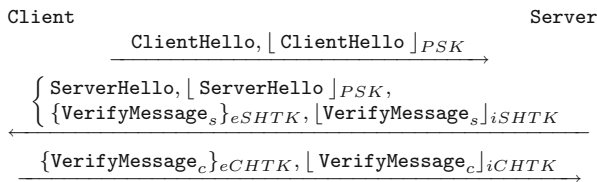
Fig. 2 Scheme of authentication using pre-shared key. Transport layer
