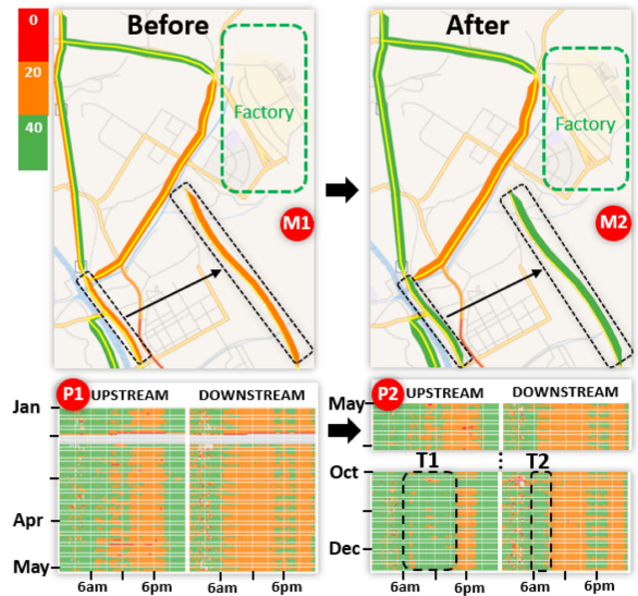
Fig. 10. Comparison of a congestion improvement project result. (M1) and (P1) present congestion conditions before the project, while (M2) and (P2) describe the result of the project. The orange road (magnified, M1) and pixels (P1) becomes green in M2 and P2.
