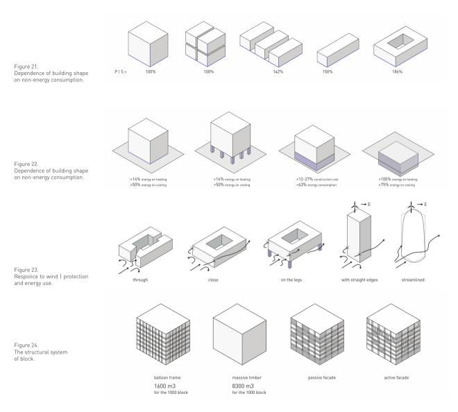
Features: The smaller the ratio between the perimeter of the building and its area, the higher the energy efficiency. Above the ground block increase the energy demand of 14% for heating and 50% for cooling in comparison with the partially underground solutions. It is necessary that the building is located end to the direction of the wind. The structural wood is much more economical and visually facilitates the construction of high-rise towers
