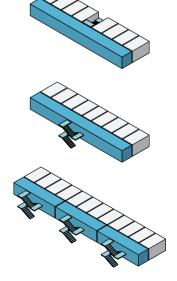
Figure 27. [left] Gallery type a. the stairs are located in the house's overall dimensions b. ladders removed from the overall dimensions of the house. c. gallery-sectional house
