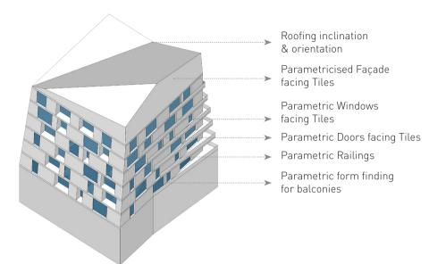
Figure 42. Parametric design application in building block.
