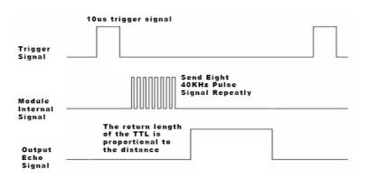
Figure 25. HCSR04 device timing diagram.
