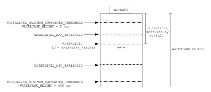
Figure 25. Water tank with its associated levels and thresholds.
