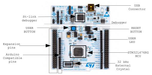
Figure 1. The Nucleo development board with the STM32L476RG MCU.
