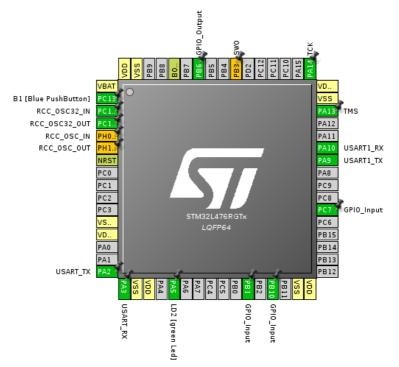
Figure 6. Microcontroller pinout configuration.
