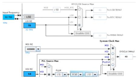
Figure 7. System clock configured to operate at 48 MHz.
