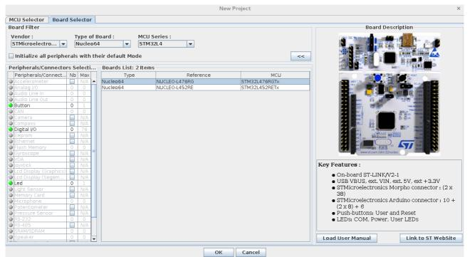
Figure 3. Microcontroller board selection on STM32CubeMX.
