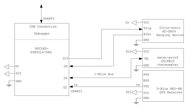
Figure 5. Connection between the MCU board and the different sensors used by the system.
